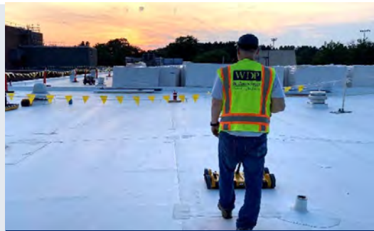
Roof Impedance Scanning
